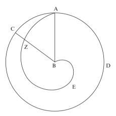
This line,<sup>3</sup> however, is called spiral. And its principal *symptoma*<sup>4</sup> is of the following sort. Whichever <straight line> is drawn through the interior toward it, such as BZ, and produced <to C>, the straight line AB is to the <straight line> BZ as the whole circumference of the circle is to the arc ADC.<sup>5</sup> This, however, is
