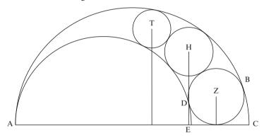
Now, that the perpendicular from Z onto AC is equal to the radius of the circle around Z, is clear. However, I say that, also, the perpendicular from H is three times the radius of the circle around H, whereas the <perpendicular> from T <is> five times <the radius of the circle around T>, and the perpendiculars in sequence <are> the multiples of the radii in accordance with the odd numbers in sequence.
